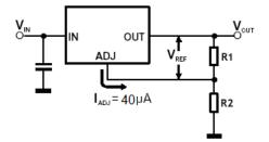
The LD6363 series develops a 1.25V reference voltage between the output and the adjust terminal. Placing a resistor between these two terminals causes a constant current to flow through R1 and down through R2 to set the overall output voltage.
